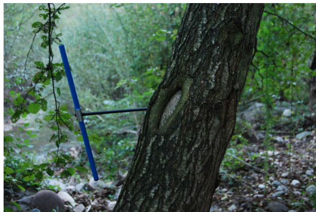
Figure 3. Dendrogeomorphological sampling in 2018 with a Pressler borer on an alder ( Alnus glutinosa ) on the banks of the Flamisell River, close to the scar caused by one flood.
